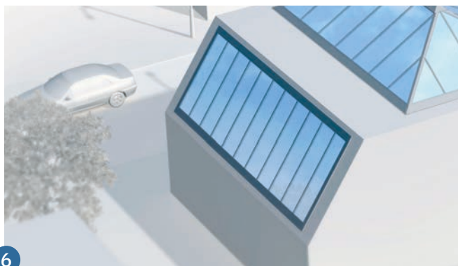
6 Mono pitched solutions Mono pitched solutions are single rows of VELUX Glazing Panels installed between 15-90° on either an upstand (on a flat roof) or a non-protruding installation in a sloped roof. Solutions mounted against a vertical wall can be installed in pitches between 15-60°.
