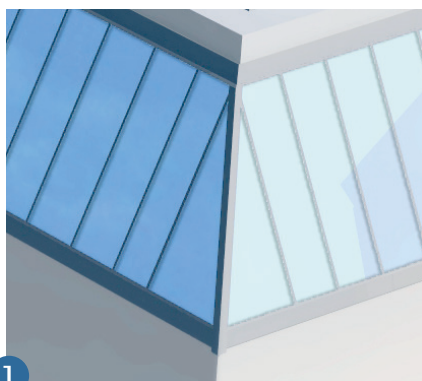
1 Hip A hip is an outward going corner solution used to connect two sloped sides. It is commonly used for making hipped gables in dual pitched solutions.
